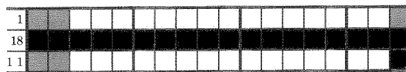
Figure 5: Contents of a 3-strip after the third sweep ( n = 18 ). Gray squares denote unknown pixels.
